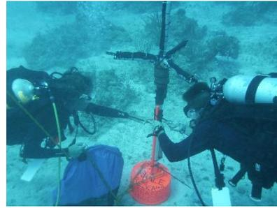
Figure 3. Acoustic recorders are being placed in strategic locations in Northwest Providence Channel to record noise generated by ships and whales for one year.
